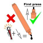
Pressure built up in the barrel by heat, usually caused by a change in ambient temperature or handling, will be released when you press down on the tip.
